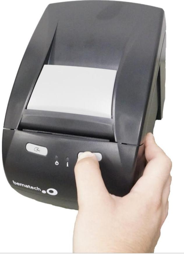
A close-up photograph of a person's hand pressing the 'Avança Papel' button on a black Bematech printer. The printer has a paper tray at the top and a control panel with a power button, an information button, and the 'Avança Papel' button. The Bematech logo is visible on the front. | <p>Com a impressora desligada. Pressione e segure o botão Avança Papel.</p>                   |
