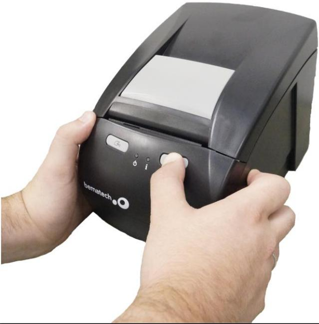
A photograph showing a person's hands holding the Bematech printer. The 'Avança Papel' button is being pressed. The printer is held at an angle, showing the front and top. The Bematech logo is visible on the front.                                                                    | <p>Com o botão Avança Papel pressionado, ligue a impressora e espere o menu ser impresso.</p> |
